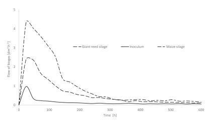
Fig. 2. Biogas flow production from individual types of input mixtures.
