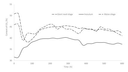
Fig. 4. Carbon dioxide content in the biogas of individual types of input mixtures.
